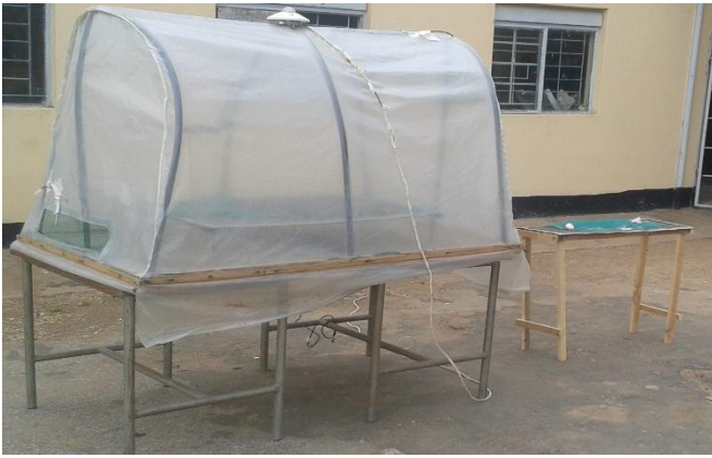
Figure. 2. Experimental drying of Kapenta inside the Greenhouse solar dryer and in open sun
